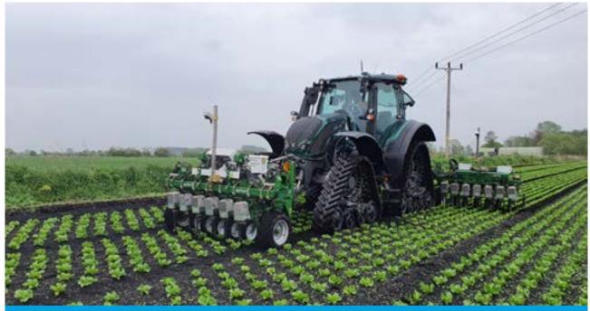
Garfords Robocrop system combines colour, infrared and depth information with AI to precisely identify plants and stem locations
