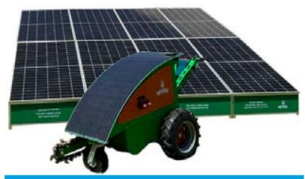
Micro Electric Tractors – Scaled to the needs of smallholder farmers, these tractors are affordable, robust, and charged directly from the microgrid
